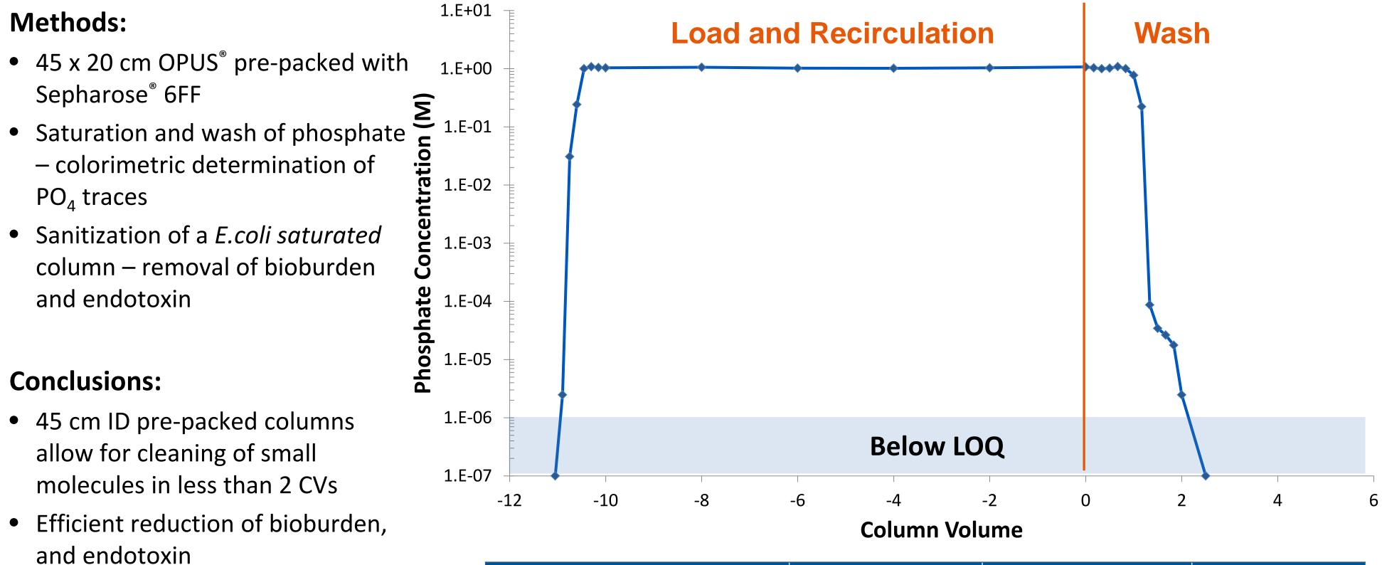
Columns are suitable for multicycle campaigns that require cleaning, sanitization and/or storage in between runs
