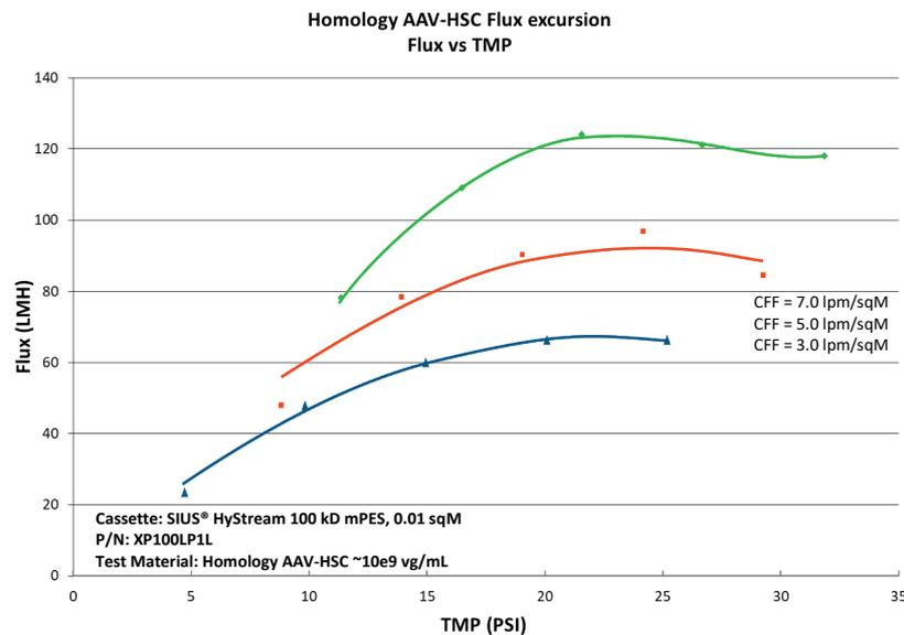
**Figure 3.** Flux excursions curves determined the optimal TMP and CFF conditions.
