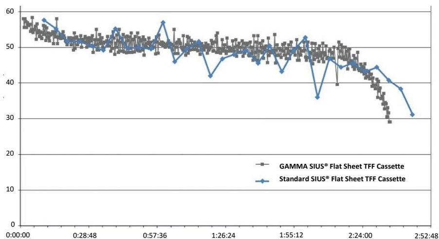
**Figure 7.** 50 X concentration of non-irradiated TangenX<sup>®</sup> SIUS<sup>®</sup> Cassette and the irradiated TangenX<sup>®</sup> SIUS<sup>®</sup> Gamma Devices.
