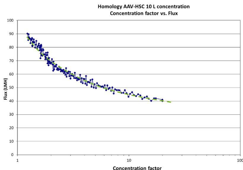
**Figure 4.** Plot of concentration versus flux during a 20 X concentration of 10 L - 0.5 L using a 0.1 m<sup>2</sup> TangenX® SIUS® Cassette.
