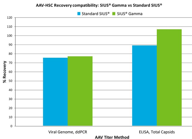
**Figure 8.** Comparison of recovery during concentration using a SIUS® Cassette and SIUS® Gamma Device.
