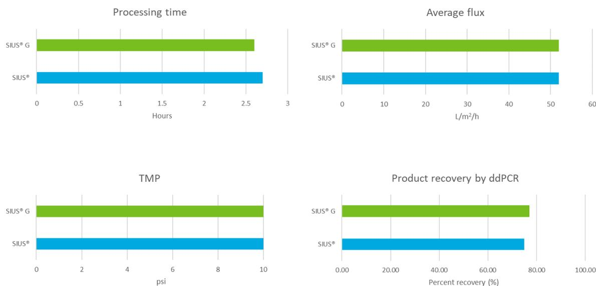
**Figure 9.** Equivalency of TangenX® SIUS® Gamma Device and SIUS® Cassettes. Process parameters for average flux, processing time, TMP and product recovery were highly comparable for the batch split processing using SIUS® and SIUS® Gamma configurations.
