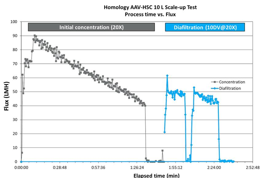
**Figure 5.** Flux tails from 90 - 40 LMH during concentration and then remains steady at 50 LMH during diafiltration. Gaps in recording indicate sampling from the product reservoir for off-line analysis.
