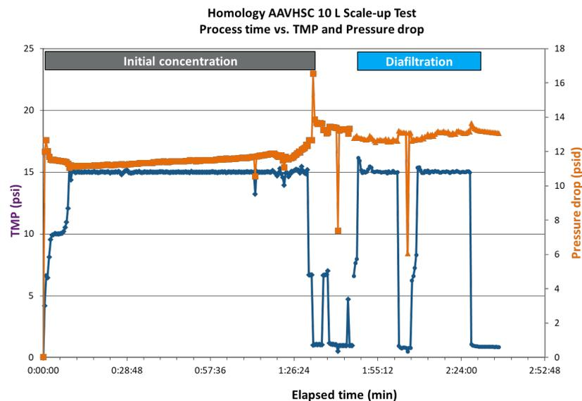
**Figure 6.** Plot of TMP versus elapsed time indicates robustness towards fouling.
