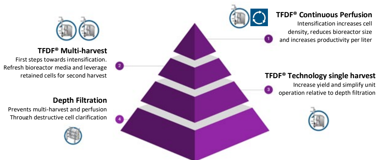
Figure 4. The progression from depth filtration to perfusion-based continuous processing. Standard depth filtration harvest process (1), TDF® single harvest (2), TDF® multi-harvest, the first step towards intensification (3) and intensification with continuous perfusion (4).
